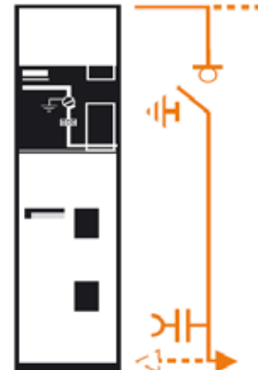
Switch unit-with/ without earthing switch -right or left outgoing line (375 mm)
